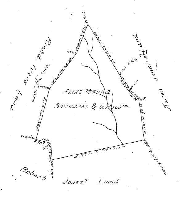
The above is the Draught of a survey made August the second 1786 on the Watters of Whitely Ball, de Hope Containing three Hundred acres together with the usual allowance of six pr. bent for roade 3c. Survey, d in pursuance of a varient granted Elias Stone June 19th. 1786
